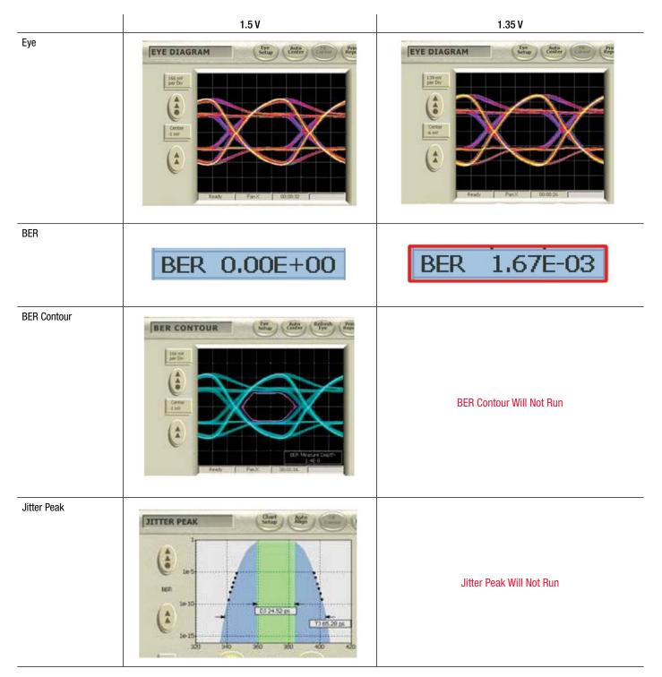
Figure 1. Operation at different supply voltages, the left column showing signal integrity measurements in the correct operating region. The right column showing measurements following the IBIST pattern generator failing. Note that the eye diagram looks identical in either case, but the BER and related measurements show otherwise.
